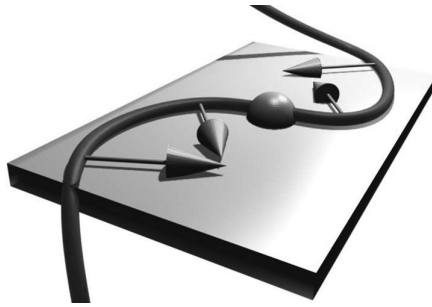
Fig. 13.20 [Colour online] A string with inflection point (ball). At each point, the Frenet-frame normal vector points towards the centre of the osculating circle. At the inflection point, we have a discontinuity in the direction of the normal vectors: the radius of the osculating circle diverges, and the normal vectors are reflected in the osculating plane, from one side to the other side of the string.
